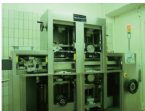
Fig.1 Presster™ as a mechanical simulator of a high speed rotary press [11]
