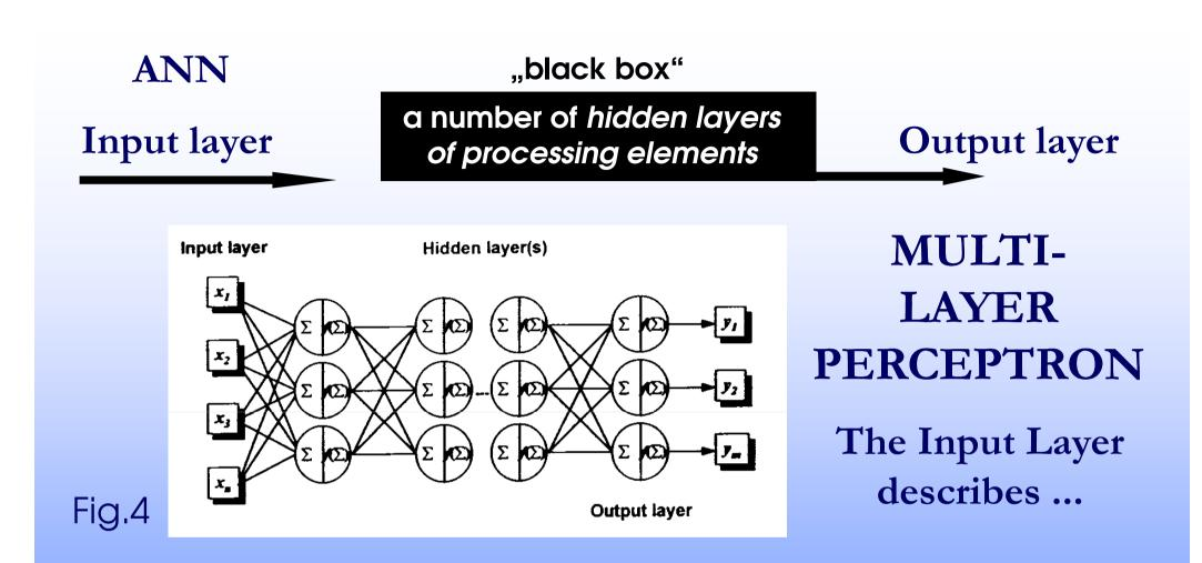
... the independent values of the variables  $x_{sm}$  (m = 1...p) fixed for a certain experiment s, which yield the output  $y_s$  (= result) in the output layer. In each processing element the sum  $z = \sum x_{sm} w_m$  is calculated to be used in the activation function and the weights are determined in order to receive an output  $y_s$ close to the target value  $t_s$ .
