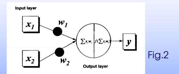
Perceptron with a single Processing Element (PE) These pulses are summed
