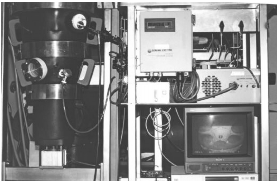
Figure 5. Atmospheric spray-freeze-drying prototype apparatus.
