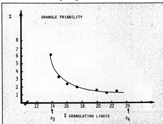
Figure 6 compares theory and experiment, i.e. the experimentally determined range of weights of granulation liquid giving satisfactory results and the calculated weights, for various tamped densities. In practically every case the calculated value lay between the two values  $S_3$  and  $S_4$ , i.e. was within the acceptable range.
