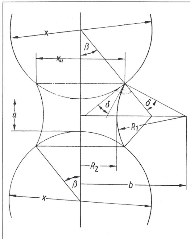
In the calculations it is important to note that even when liquid bridge formation is minimal the cohesive force rises steeply, passes through a maximum, and slowly falls as the liquid bridges become progressively larger. In this case when, after an initial wetting phase, the first bridges are formed throughout the powder mass. A large build-up of cohesive force must occur, leading to the marked increase in power consumption seen in Figure 2.
