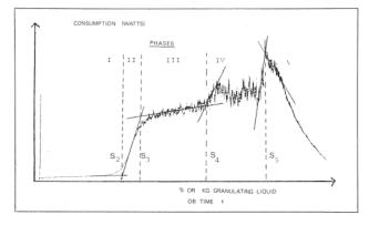
These five phases were obtained with practically all the compositions investigated. As Figure 3 indicates, changing the type of mixer also has only a slight effect on the phases of the kneading process. However, the actual power consumption of mixers of different type (Glen planetary mixer, Meili Z-blade mixer) differs greatly for a given granulate composition. Nevertheless, kneading phases 1–3 which are important in practice are clearly recognizable with
