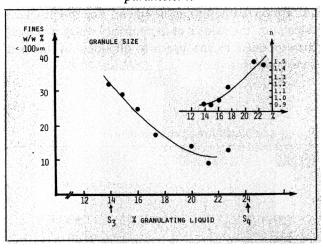
Figure 9 Resistance of the granulates to abrasion
