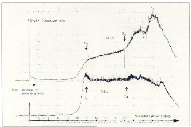
Figure 4 Scale-up precision measurements with identical charges
