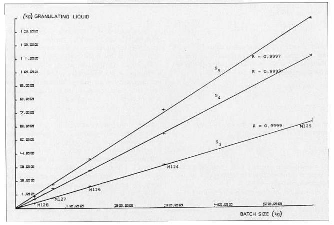
both machines. Furthermore, the power consumption curve, as defined by the parameters  $S_3$ ,  $S_4$  and  $S_5$ , is also independent of batch size (Fig. 4). It may then be asked whether a theoretical explanation can be found for this evidently quite generally valid power-consumption curve.
