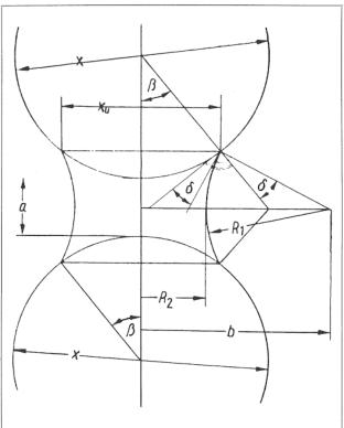
In the calculations it is important to note that even when liquid bridge formation is minimal the cohesive force rises steeply, passes through a maximum, and slowly falls as the liquid bridges become progressively larger. In this case when, after an initial wetting phase, the first bridges are formed throughout the powder mass. A large build-up of cohesive force must occur, leading to the marked increase in power consumption seen in Figure 2.
