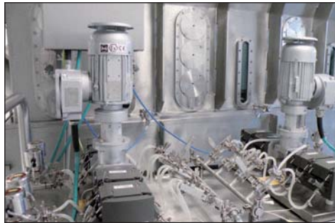
Level 1: ProCell 250 Inlet air chambers and process chamber (LH), trolley with spray pumps (RH)
