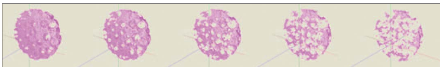
Figure 4. From left to right: Reduction of a porous network (pores depicted as pink) during growth of solid particles (solids are transparent).
