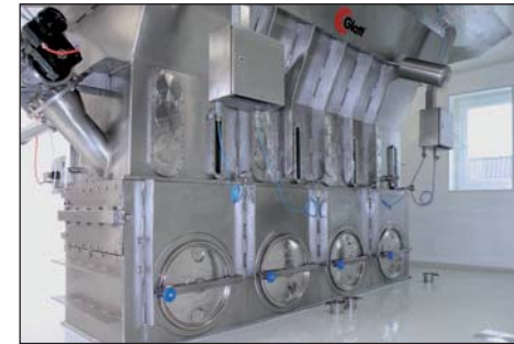
Level 1: ProCell 250 Inlet air chambers and process chamber (LH), trolley with spray pumps (RH)
