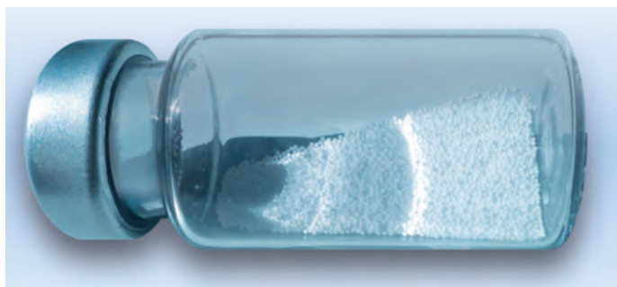
Fig.1.3: Vial with mono-sized pellets obtained by Spray Freeze-drying. (Courtesy Meridion)
