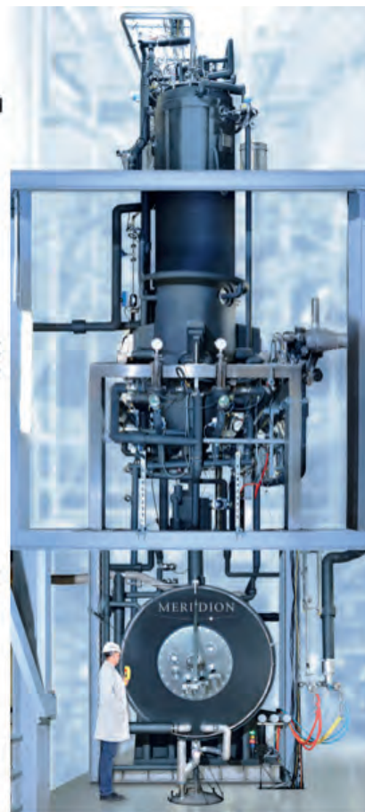
Fig.2.4.2: Industrial Spray Freeze-drying Concept for Aseptic (full containment) Processing. (Courtesy Meridion).
