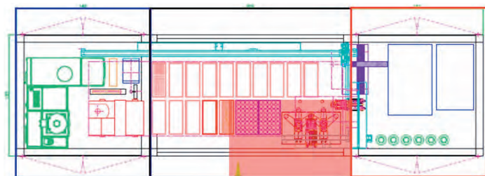
Fig. 7: Automated system for physical and chemical stability testing. The system consist of a set of racks (middle) for the storage of up to 1000 test samples under controlled conditions (temperatrue., humidity), several devices for non-destructive physical (camera, near infrared & Raman spectroscopy (left side)) and chemical (UPLC/MS, (right side)) analysis after automated sample preparation (red-colored area).
